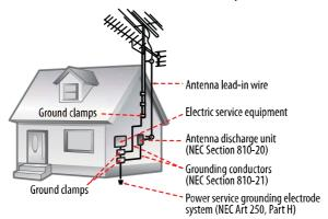
regard to proper grounding of the mast and supporting structure, grounding of the lead-in wire to an antenna-discharge unit, size of grounding conductors, location of antenna-discharge unit, connection to grounding electrodes, and requirements for the grounding electrode (see figure).
