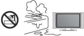
Keep the LED TV away from any heat sources or direct sunlight. To ensure good ventilation, allow 10 cm. between the LED TV and other appliances or built-in cabinet walls.
