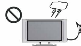
Unplug the power cord and antenna cable during electrical storms to prevent damage to the LED TV from electrical surges. Keep clear of the antenna cable during electrical storms.
